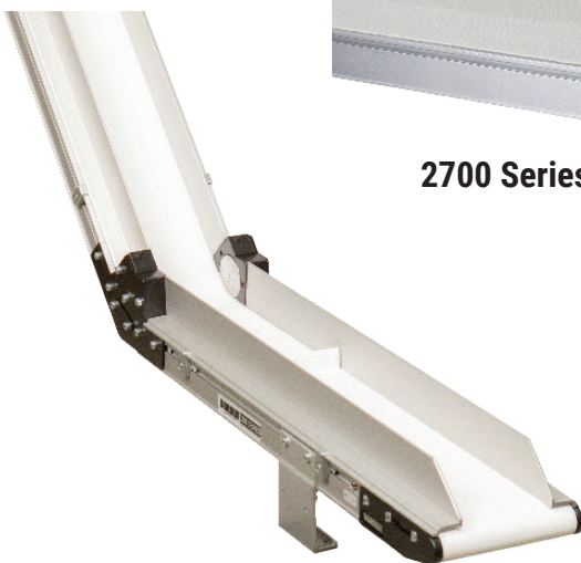
Horizontal to Incline
